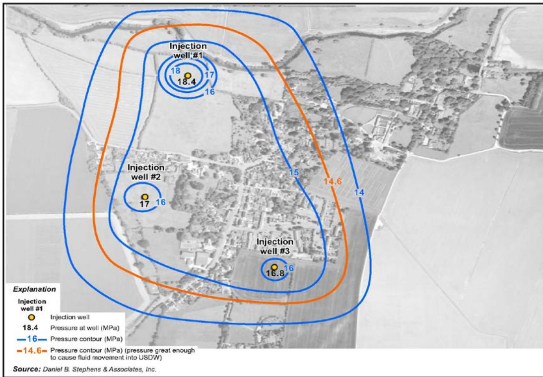
Figure 3-4: Hypothetical Geologic Sequestration Site: Model Predicted Maximum Pressure Within the Injection Zone.
